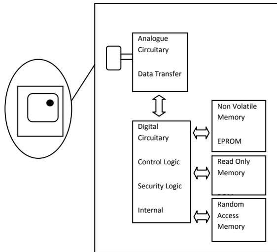
to temporarily hold incoming data following demodulation and outgoing data for modulation and interface with the transponder antenna. The interface circuitry provides the facility to direct and accommodate the interrogation field energy for powering purposes in passive transponders and triggering of the transponder response.
