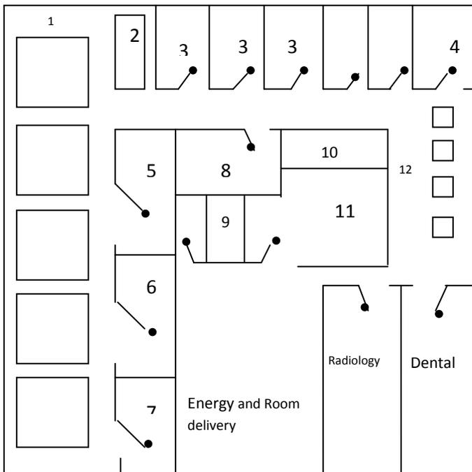
● Indicates RFID location in a sample hospital plan
